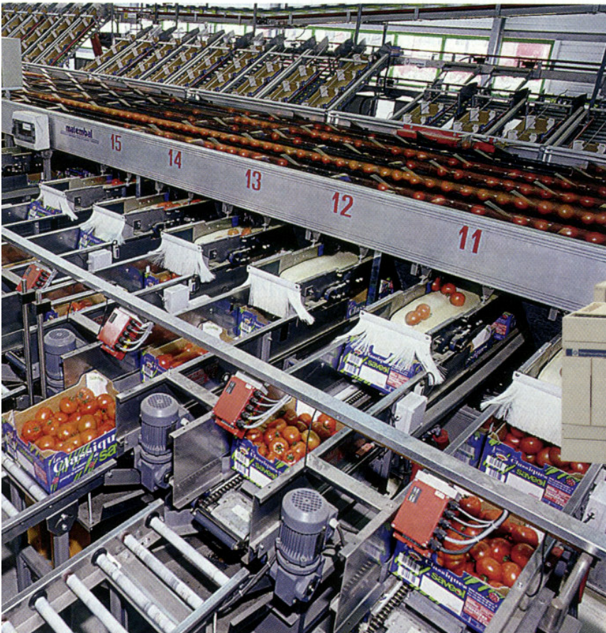
Telemecanique Twido Nano PLC from Schneider Electric controls these conveyor and packaging lines in a fruit and vegetable plant.
