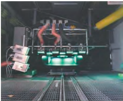
The Team UV racecar project used many fixed lamps to cure a small UV-coated racecar.
