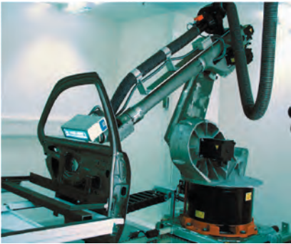
The Daimler-Chrysler UV Technology Center in Ulm, Germany, tests robotic cure.
