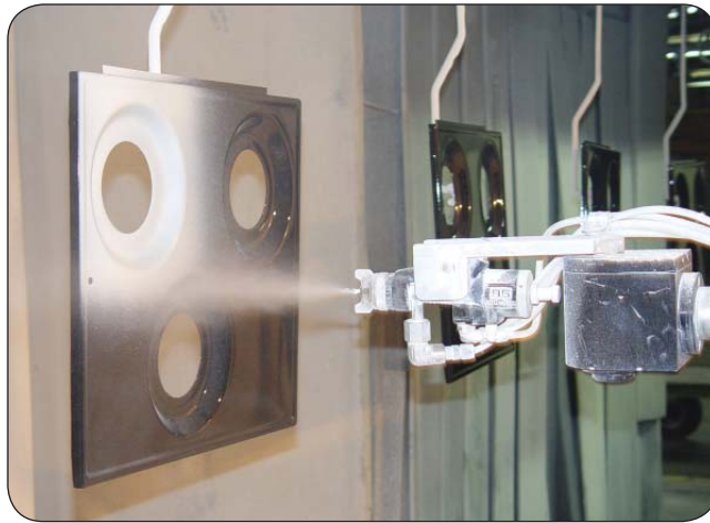
The introduction of robotics to PMC’s facility has saved the company 40-60% on wet enamel usage.
