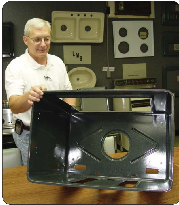
Oven cavities, like the one demonstrated here by Quality Director Frank Zebich, are representative of the type of porcelain enameling work done at Porcelain Metals Corporation
